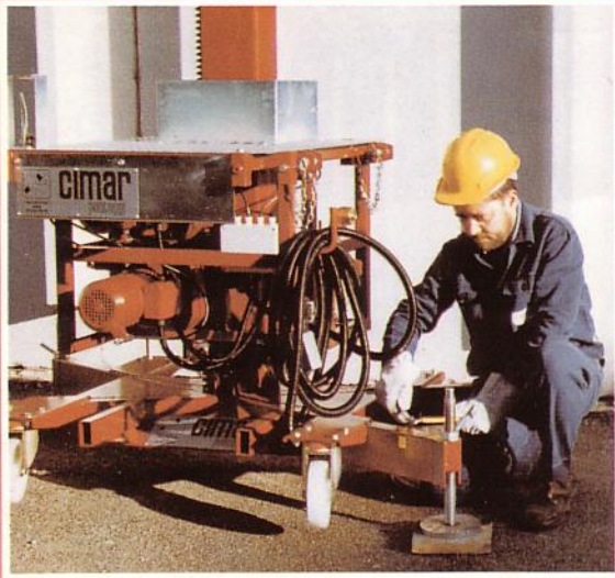
Basement and drive platform on castoring wheels.
