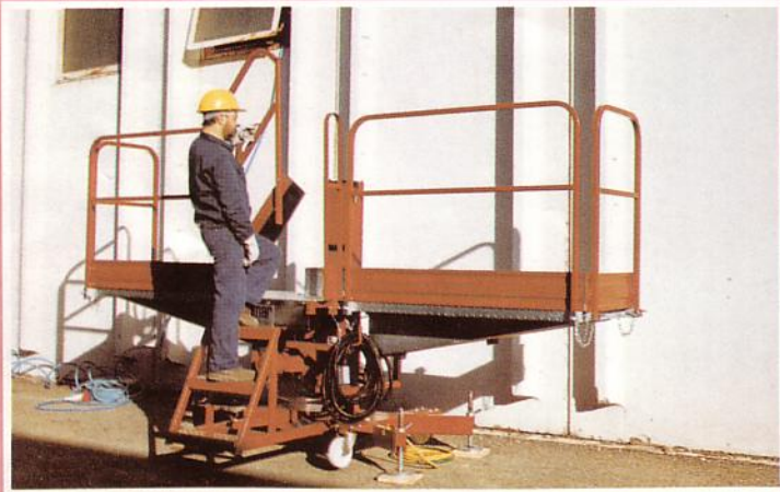
Access to deck area and total protection also during erection.
